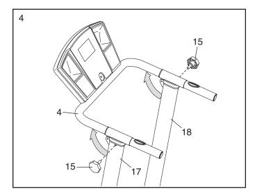
5. Pivot the console assembly to the desired position, and tighten the two Console Knobs (3).
